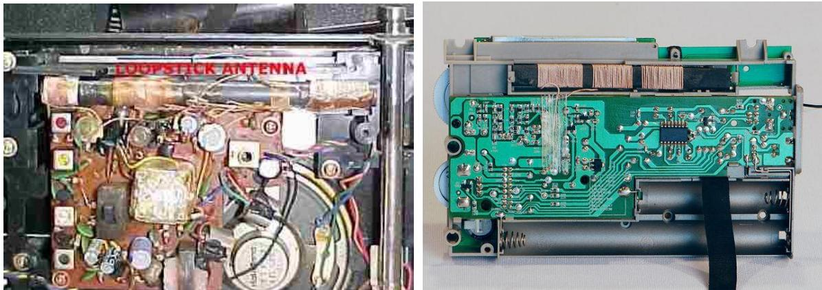
How they work is that any loop of wire has a magnetic field. When that magnetic field picks up the magnetic field energy lines from the transmitter signal, some of that energy is converted into electricity and fed into the radio amplifier circuits.
